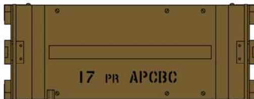
17 Pounder Ammunition Case C310 Mk.I (wood) containing 2 rounds of A.P.C.B.C.
