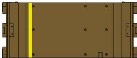
17 Pounder Ammunition Case C274 Mk.I (wood) containing 2 rounds of A.P., A.P.C., H.E. or Practice (yellow band denotes)
